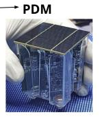
**SPADs - Single Photon Avalanche Diodes**: semiconductor devices based on a p-n junction, reverse biased well above breakdown voltage (operating in Gieger mode).
