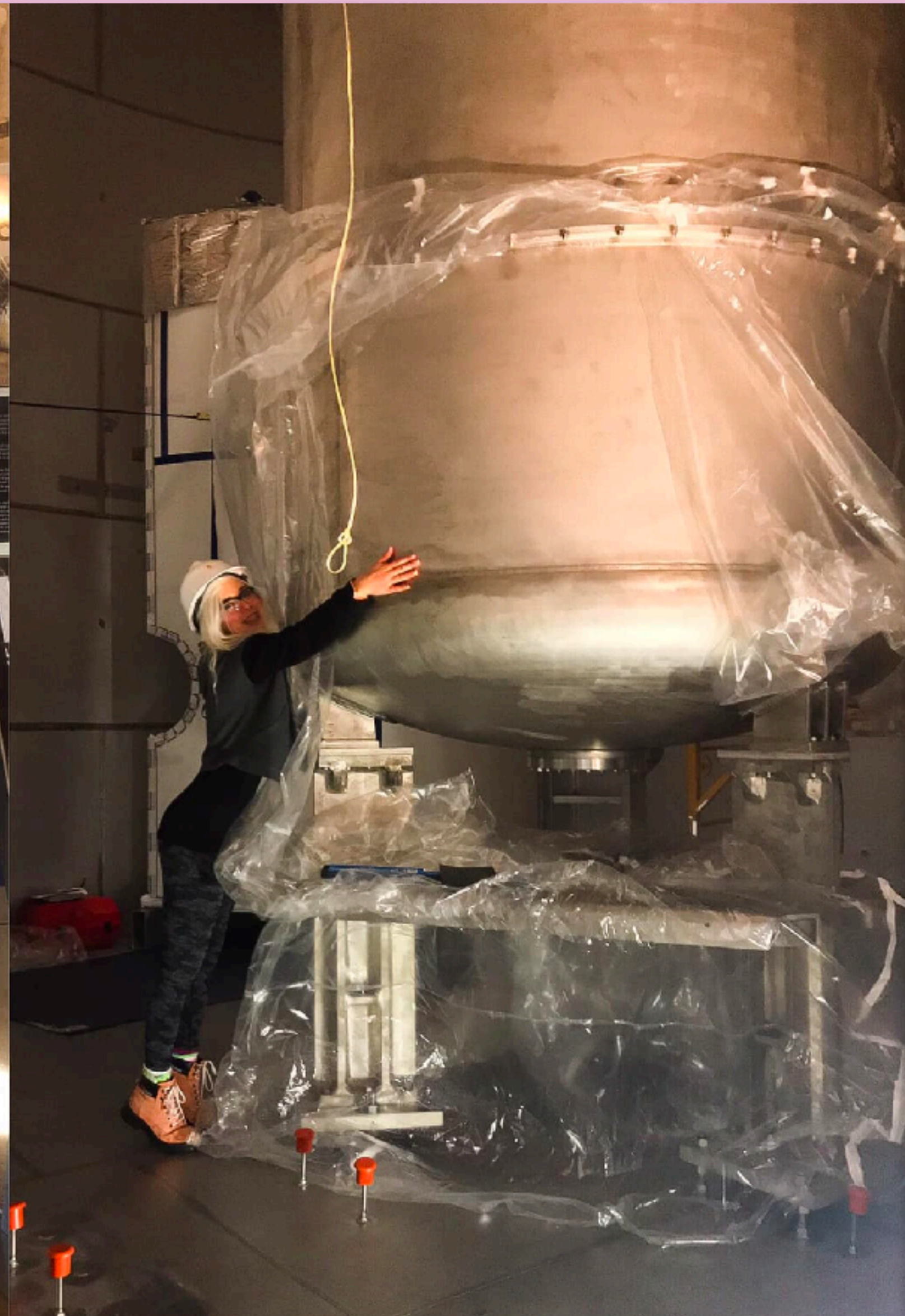
LZ Outer Cryostat
