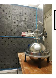
Investigate the capability of the SPC to detect fast neutrons and neutrons thermalized by the graphite.
