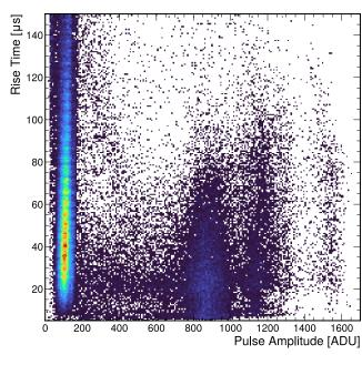
Confirmation of thermal neutrons peak from <sup>222</sup>Rn decay peaks
