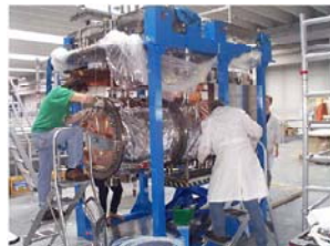
Al prototype and the final installation of the superconducting RFQ at LNL, Italy
