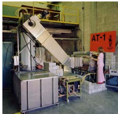
Proof of Principle (POP) RFQ, Los Alamos 1980 – the 1 st vane-type RFQ 100 KeV - 650 KeV, 30 mA , 425 MHz
