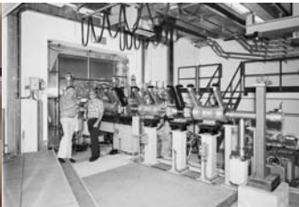
The old pre-injector at CERN (1976): Source+ Cockroft Walton +line+bunching
