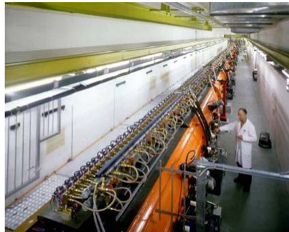
Top; CERN Linac2 Drift Tube Linac accelerating tank 1 (200 MHz). The tank is 7m long (diameter 1m) and provides an energy gain of 10 MeV. Left: DTL prototype for CERN Linac4 (352 MHz). Focusing is provided by (small) quadrupoles inside drift tubes. Length of drift tubes (cell length) increases with proton velocity.
