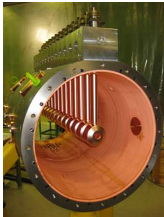
Top; CERN Linac2 Drift Tube Linac accelerating tank 1 (200 MHz). The tank is 7m long (diameter 1m) and provides an energy gain of 10 MeV. Left: DTL prototype for CERN Linac4 (352 MHz). Focusing is provided by (small) quadrupoles inside drift tubes. Length of drift tubes (cell length) increases with proton velocity.
