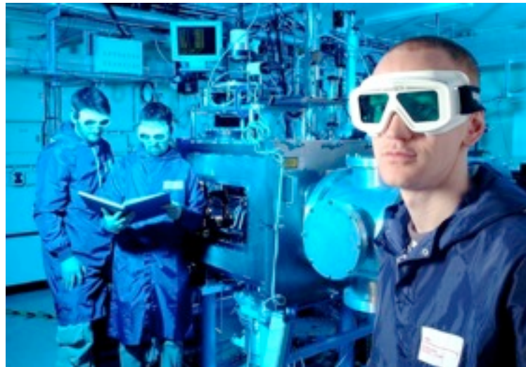
Astra laser: 500mJ at 40 fs (12 TW) (monoenergetic pulses)
