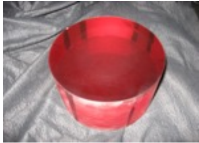
192 mm dia. Ti:Sa crystal (image courtesy Crystal Systems)
