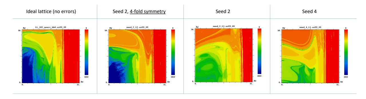
There is no damping and no noise in these simulations. The color (logarithmic scale) shows how many turns the particle made before death. Dark blue color – for particles that survived after 1012 turns. Dark red – for particle died at the 1st turn.
