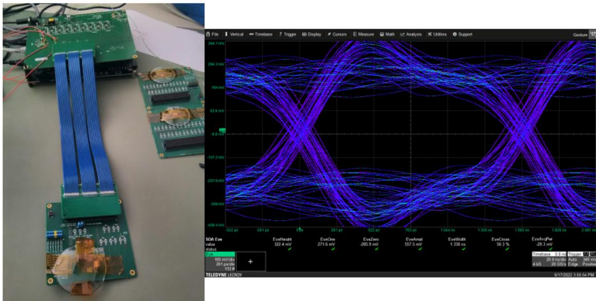
**Figure:** Left, PCB with wire-bonded chip (bottom) and common test system (top). Right, eye diagram at 640 MHz (preliminary). Acknowledgment: Giulio Borghello, Davide Ceresa, Francisco Piernas Díaz, Risto Pejasinovic.
