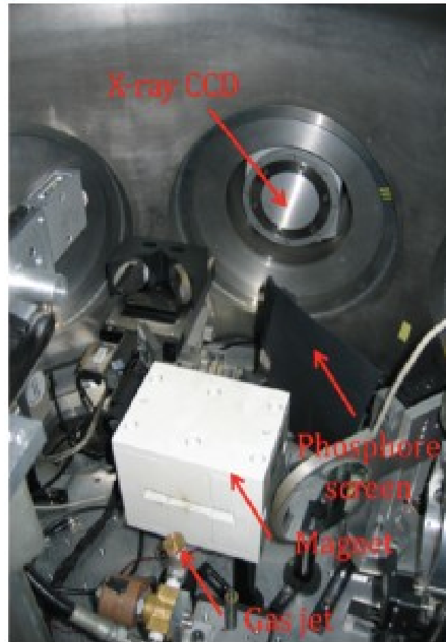
Figure 2: Left: the experimental set-up for the Betatron-based emittance measurement. It combines a X-ray angular profile measurement realized with a X-ray CCD located on axis, and an electron spectrometer composed of a magnet and a phosphor screen imaged onto a visible CCD camera. Right: an example of X-ray angular profile measured with this set-up.
