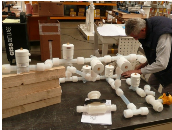
fluid distribution valves (PFA)
