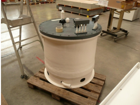
acid tank with teflon inner coating
