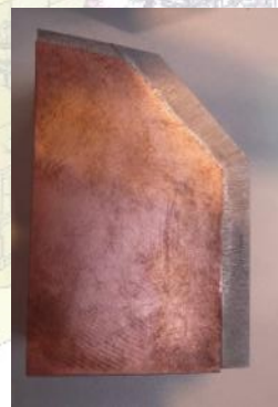
Prototype for brazing (W-Cu) technique validation
