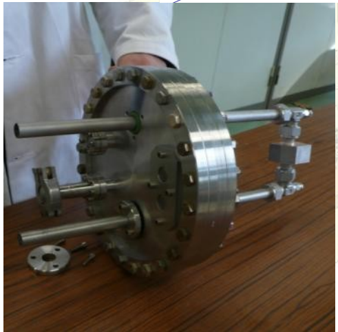
Prototype for brazing (W-Cu) technique validation
