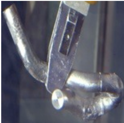
Targetry: High-intensity beam on a solid target (Ta)
