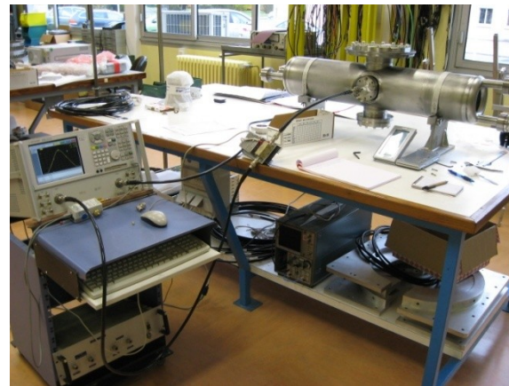
First cavity prototype under RF measurements
