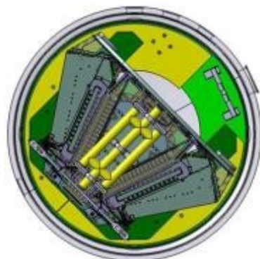
Cold mass R3B-GLAD placée inside the W7X for cold tests
