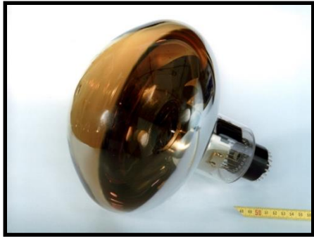
Hamamatsu PMT : Size :10 inch
