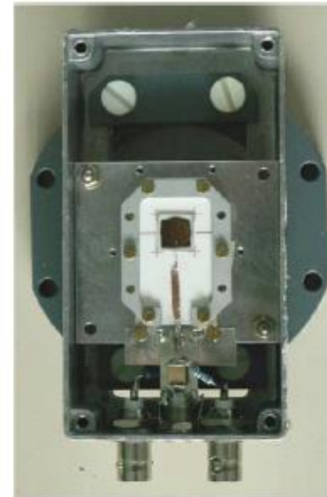
Fig. 13. The pcDD set used in a ^{181}\text{Ta} beam of 1 A GeV (left). The time difference spectrum measured between two identical detectors (right). The time resolution is 22 ps.
