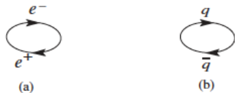
Fig. 6.29. Diagrams of the vacuum polarisation by (a) a positron–electron pair, (b) a quark–antiquark pair.
