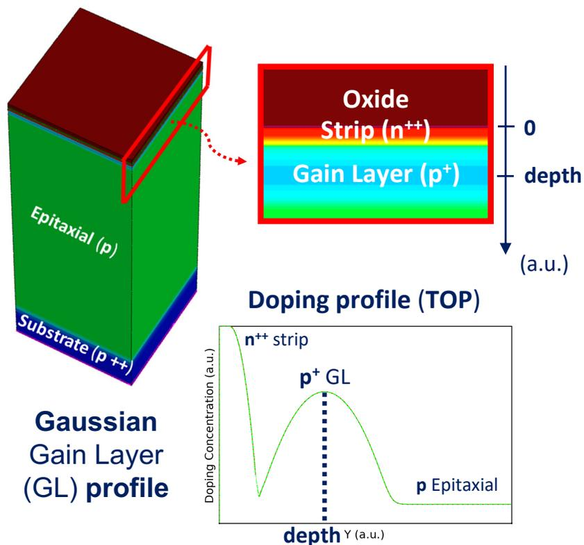
The *Heavylon* function is activated in Sentaurus to emulate an ion travelling through the detector to study charge multiplication with the passage of a charged particle
