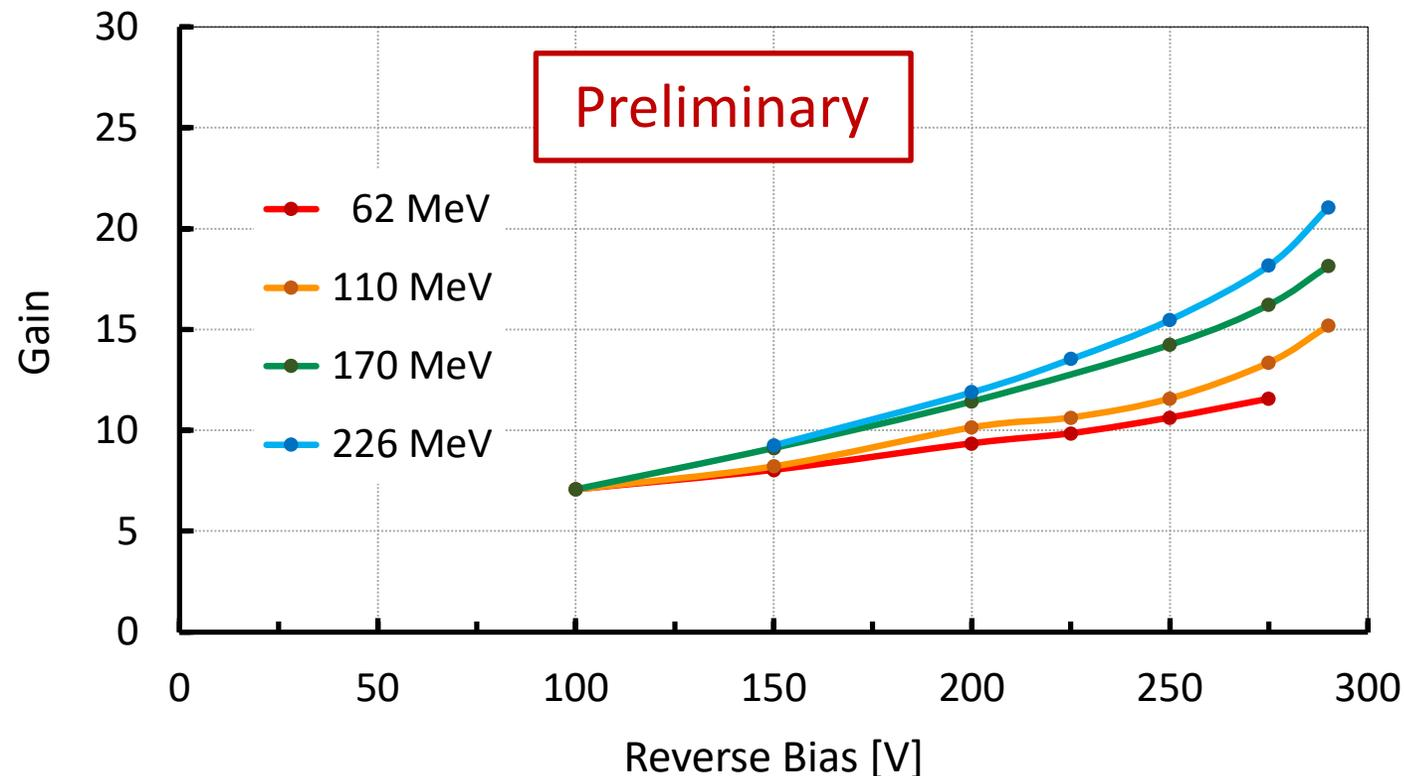
→ A gain reduction is observed with decreasing proton energy
