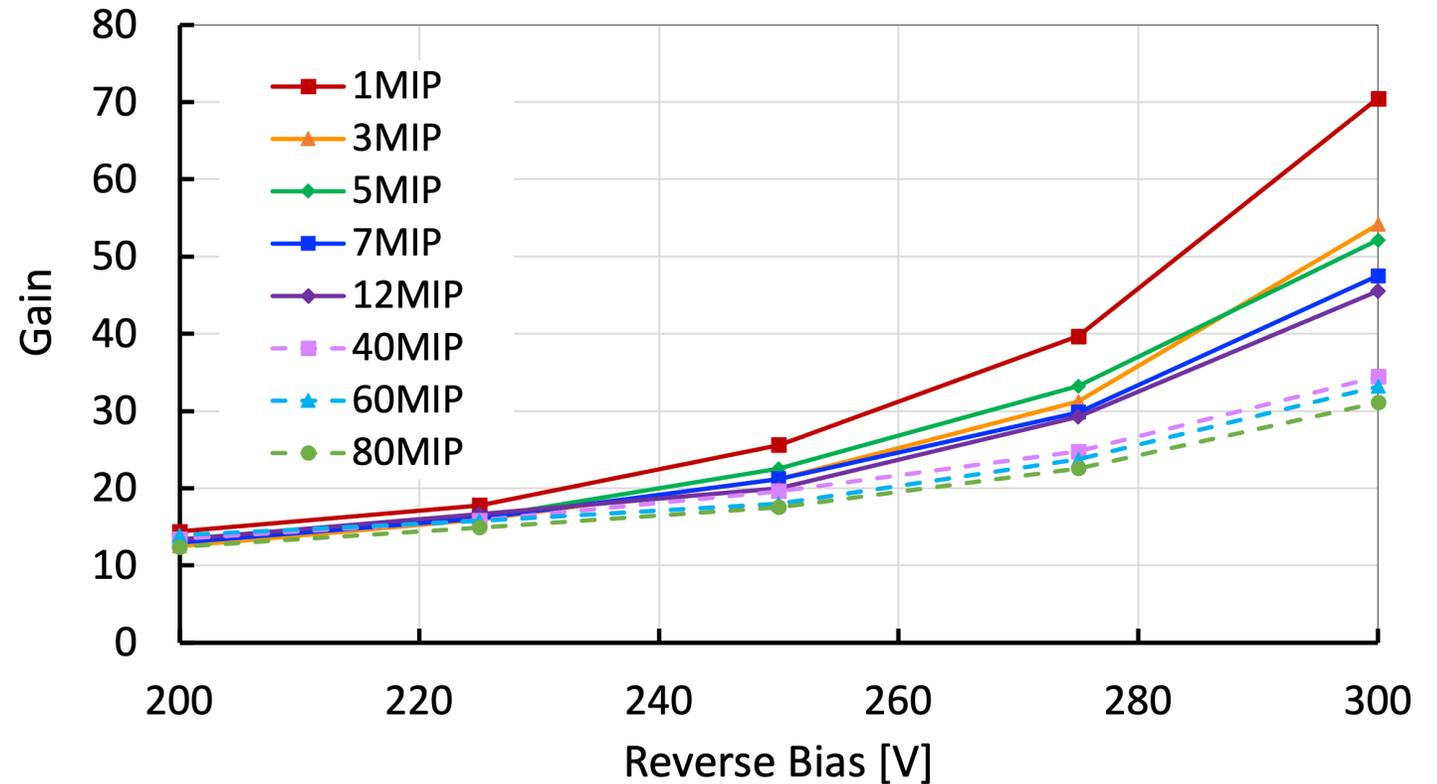
→ More than 50% of gain suppressed going from 1 to 80 MIPs
