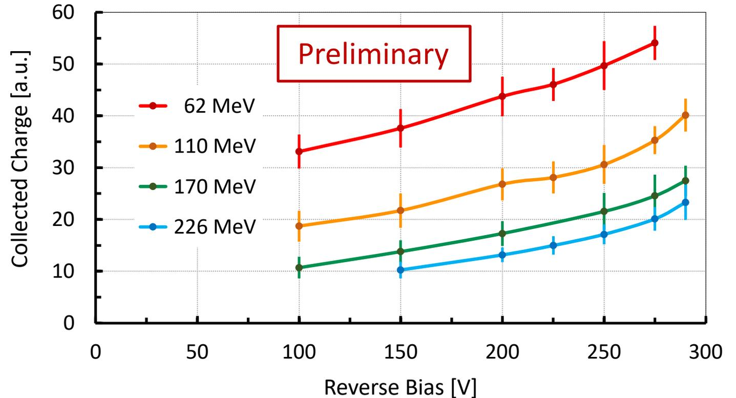
→ Collected charge scales with the impinging proton energy
