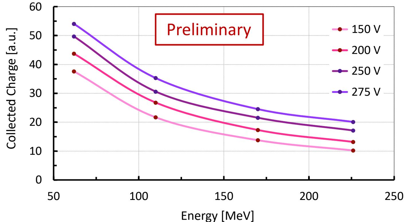
→ At fixed  $V_{\text{bias}}$ , the collected charge scales with the energy
