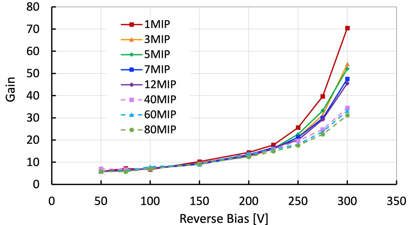
→ Suppression of gain enhanced for laser intensity  $\geq 40$  MIPs
