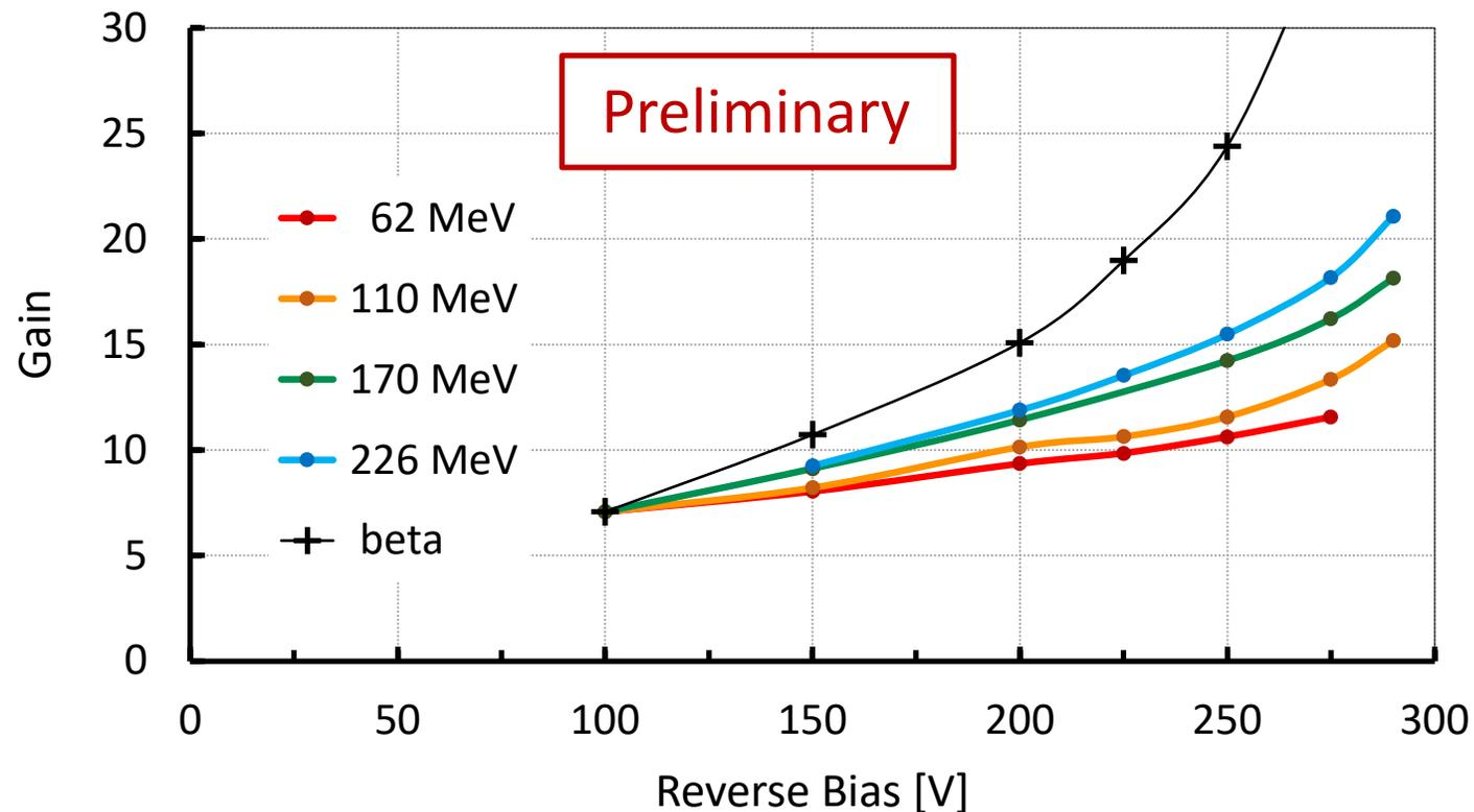
→ Gain reduction is more pronounced if compared to  $\beta$  particles
