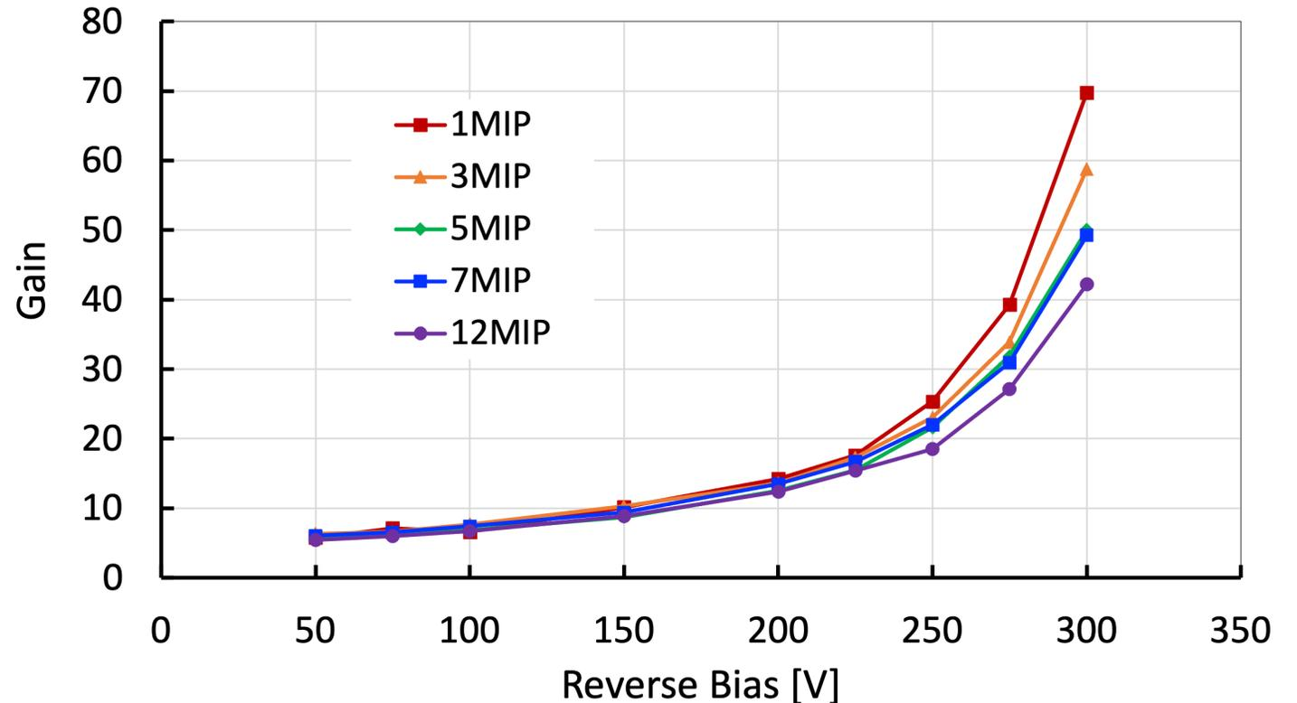
→ Gain suppression mechanism observed above 200 V
