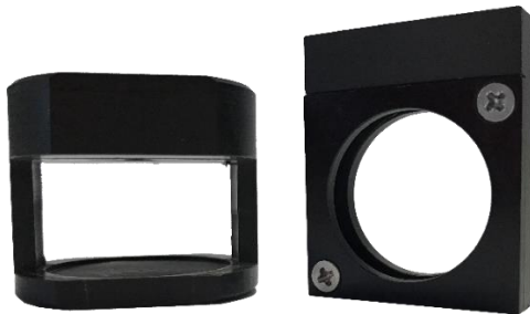
Fig. 5.5: Plastic holders allow horizontal and vertical source position
