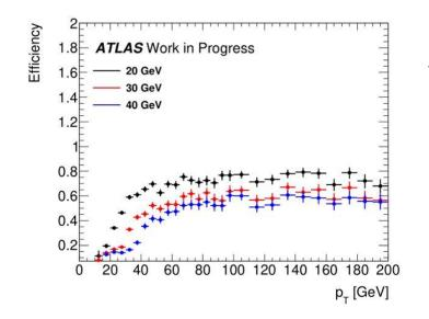
Trigger efficiency as a function of the 4th jet  $p_T$  for different trigger thresholds
