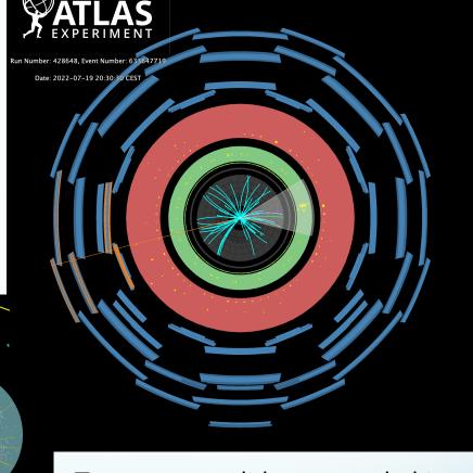
Z to e+ e- candidate recorded in ATLAS on 5 July 2022, when stable beams of protons at the energy of 6.8 TeV per beam were delivered to ATLAS for the first time by the LHC
