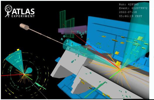
Dilepton ttbar candidate recorded in ATLAS on 18 July 2022 when stable beams of protons at the energy of 6.8 TeV per beam were delivered by the LHC
