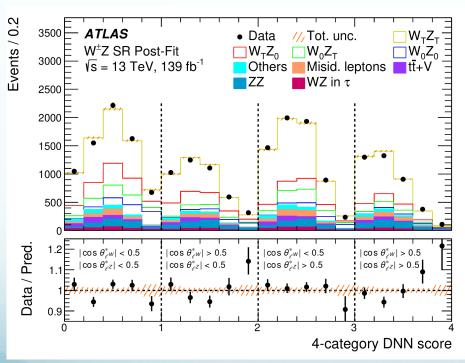
A multivariate discriminant is used to better separate the four joint helicity states. A deep neural network (DNN) classifier is implemented to exploit kinematic differences between polarisation states in different observables
