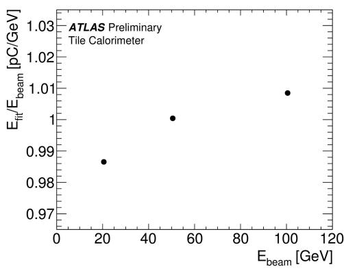
The linearity of the calorimeter response to electrons was checked in the range of 20-100 GeV. Further investigation is ongoing.
