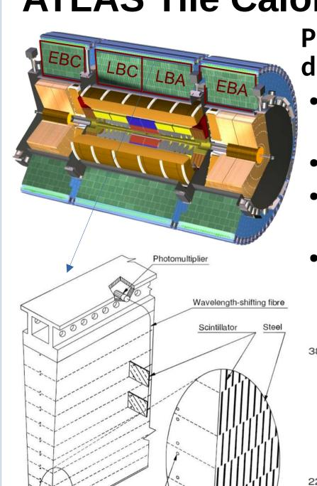
Principle of Tile Calorimeter [1] – hadronic calorimeter of the ATLAS detector
