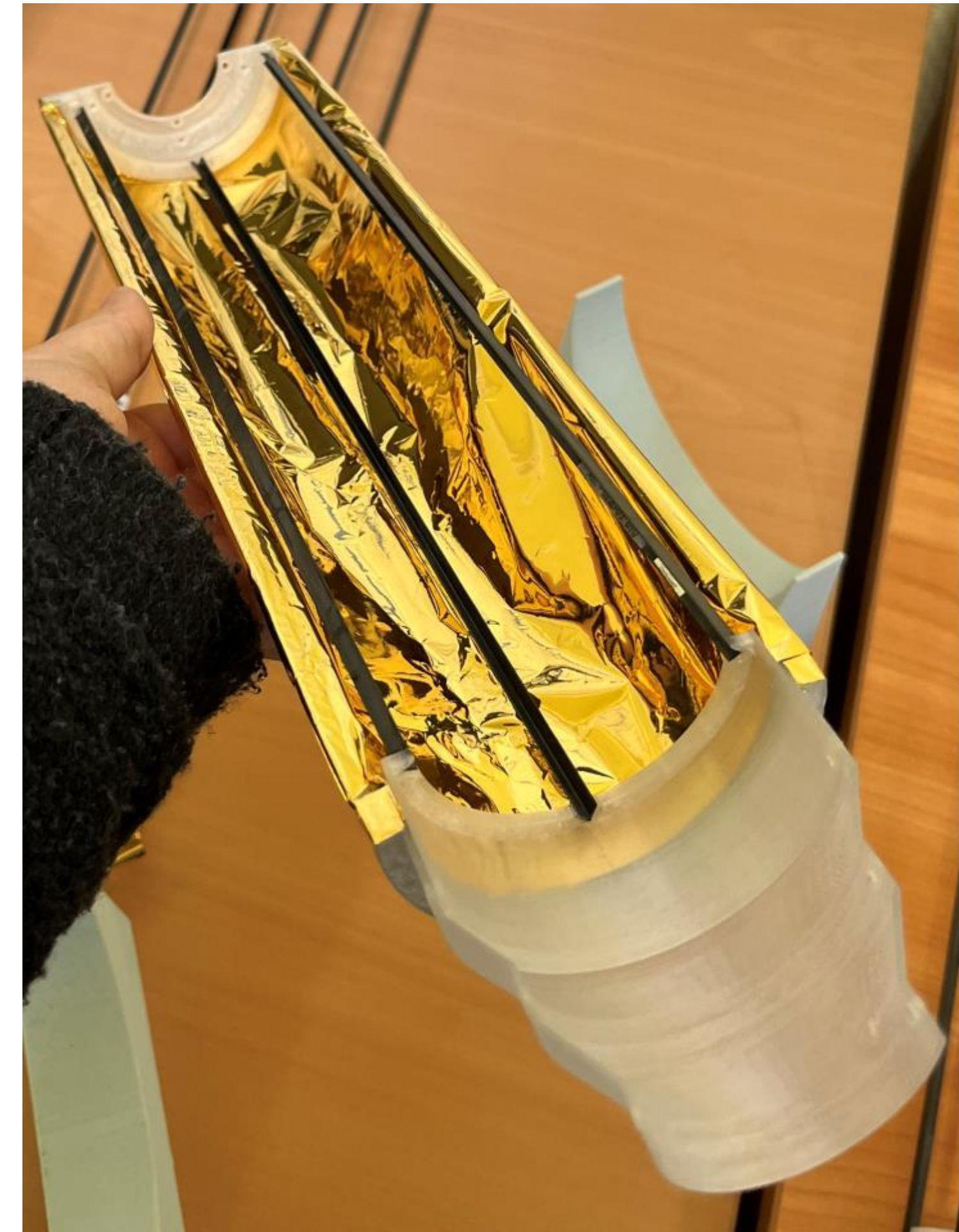
Outer shell + space blanket + 3d layer
