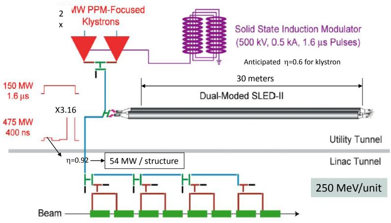
Eight 0.6 m Accelerator Structures (65 MV/m Unloaded, 52 MV/m Loaded)
