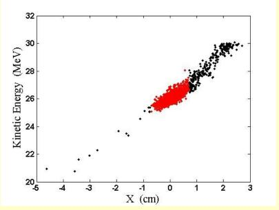
Longitudinal phase space after the cleaning chicane, 24 % intensity loss at the chicane
