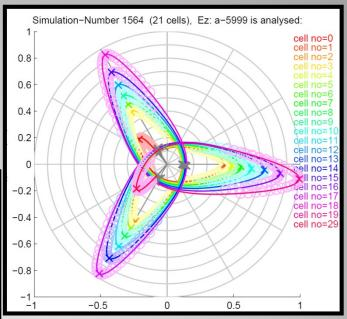
GdfidL time domain simulations to verify dipole mode damping and detuning are ongoing.
