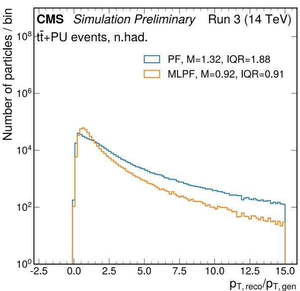
Slight improvement in charged and neutral particle p<sub>T</sub> resolution
