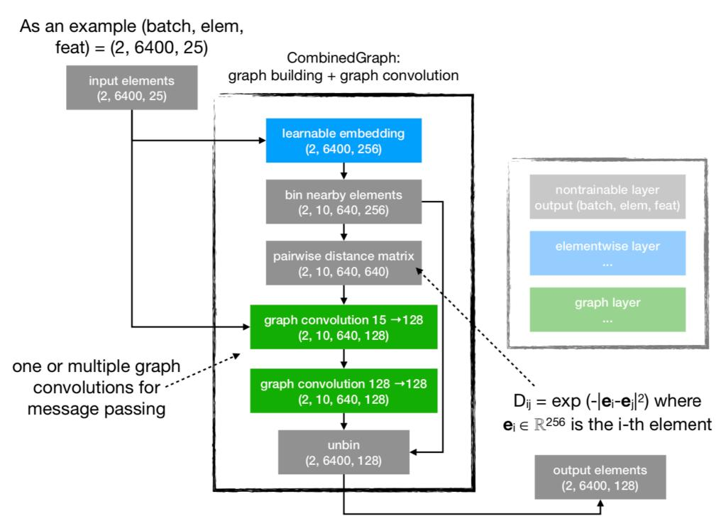
Uses built-in dense matrix, reshape and scatter/gather operations in TF. Requires batch-mode graphs. No N<sup>2</sup> allocation or computation needed.
