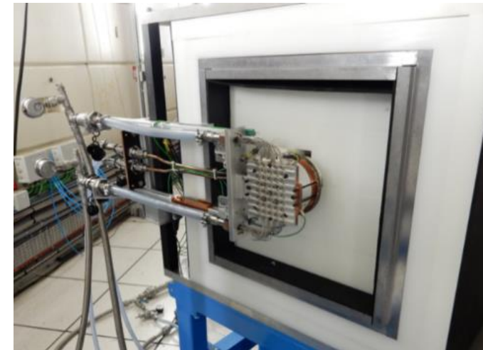
Beryllium target + cooling inside ½ moderator + shielding
