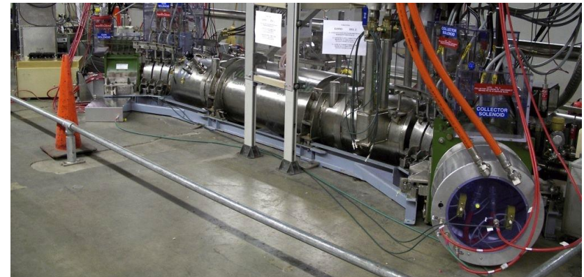
Pulsed electron lens TEL-2 at the Tevatron (Fermilab)
