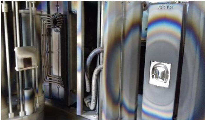
A sample and a Nb target in deposition facility at University Siegen.
