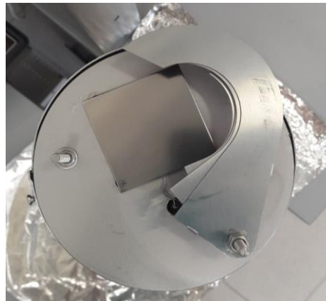
A sample and sutter assembly for the Nb deposition at LNL/INFN
