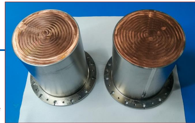
Cu-Nb samples at HZB after production
