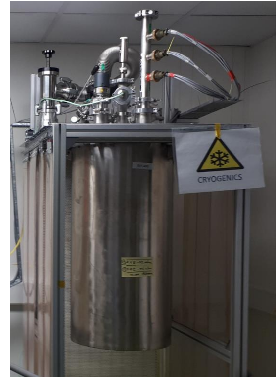
Pill-box cavity in a new facility with a closed-cycle refrigerator in STFC
