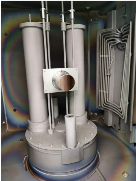
A QPR sample inside the deposition chamber at Siegen Uni. Courtesy of M. Vogel
