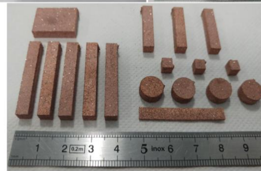
Figure 4 – Top left: 36 samples of CerGr. Top right: CuCD plate with samples cut by water-jet. Bottom: 17 samples of CuCD extracted from the plate. All specimens are for thermophysical characterization at the CERN-EN-MME Mechanical Laboratory.
