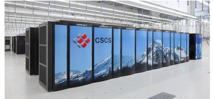
Cray XC-30 Hybrid Piz Daint at CSCS (5,272 GPUs)
