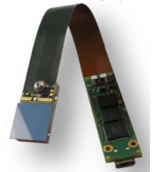
Prototype FLEX MiniPIX TimePIX3
