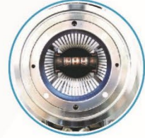
COLLIMATORS 20 novel low impedance collimators for beam stability and further 24 new collimators for improved machine protections
