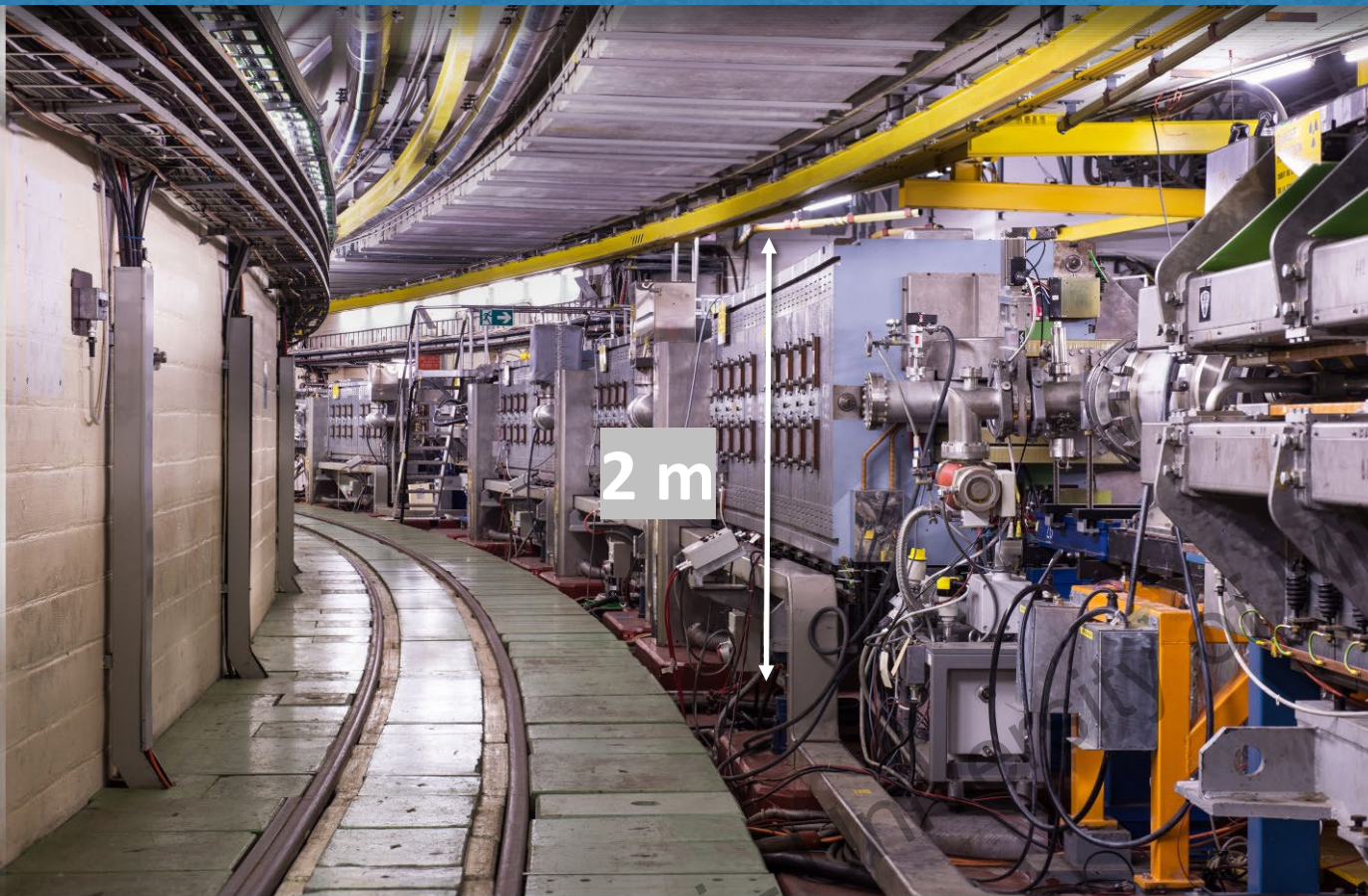
Resistive magnets of PS accelerator at CERN (1.5 tesla)
