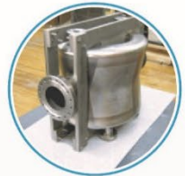
“CRAB” CAVITIES 8 SRF «crab» cavities on each side of ATLAS and CMS experiments to tilt beams at collision.
