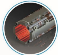
BEAM SCREEN All new magnets will be equipped with a new special beam screen to intercept collision debris at 80 K temperature and cancel electron-cloud effects.
