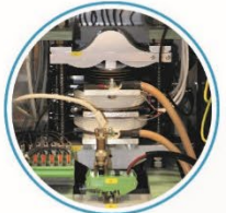
CLIQ A novel concept of magnet protection, based on fast injection of oscillating currents, will improve the safety of the very large stored energy quadrupoles.
