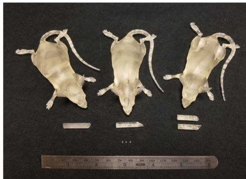
Fig. 3. Examples of mouse phantoms: the torso, with thermoluminescent dosimeters insert, is shown on the left with the head in the center and the flank on the right. Note the 1 mm cube thermoluminescent dosimeters that are put in the inserts shown under the phantom.
