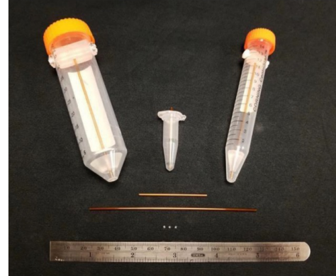
Fig. 1. Cell culture phantoms shown with the 1 mm × 1 mm × 1 mm cube thermoluminescent dosimeters shown. The Kapton inserts are shown above the thermoluminescent dosimeters.
