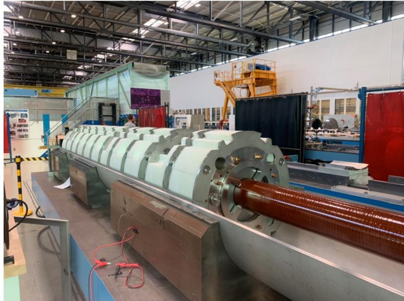
Sequence of higher order corrector magnets and preassembled cold mass of the Corrector Package [CP]
