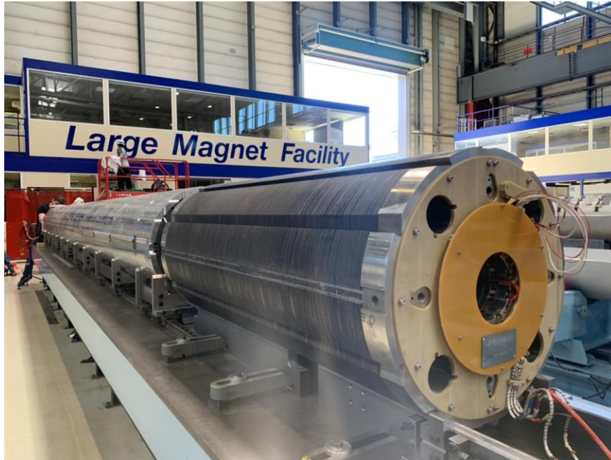
MQXFBP2 on assembly bench with nested corrector MCBXFBP1 (H. Prin, et al.)
