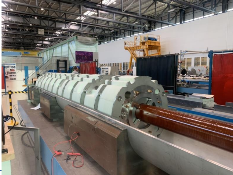
The nine high order correctors assembled in the prototype cold mass (M. Statera, E. Gautheron, H. Prin, et al)
