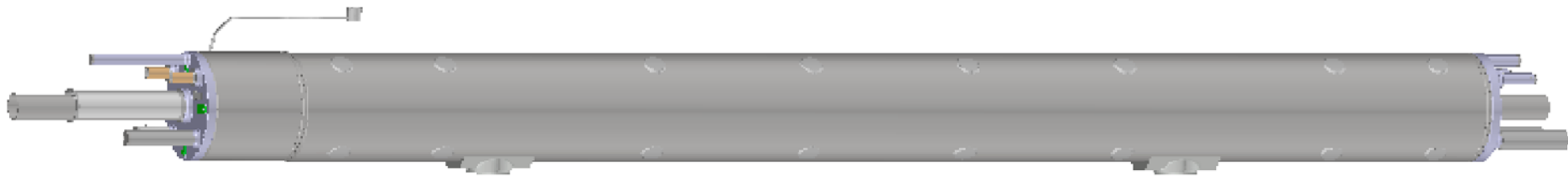
D1 magnet for vertical cold test (Yoked magnet w/ shell, end-ring)
