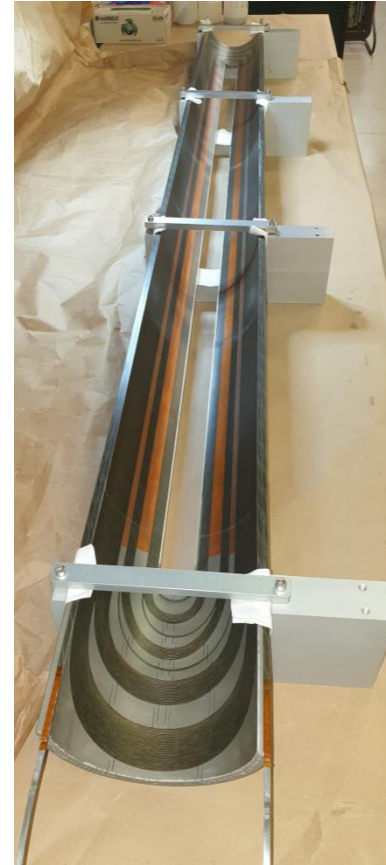
First finished inner coil
