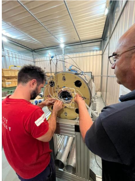
Current lead routing
