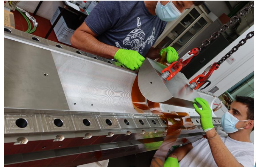
Impregnation mould assembly
