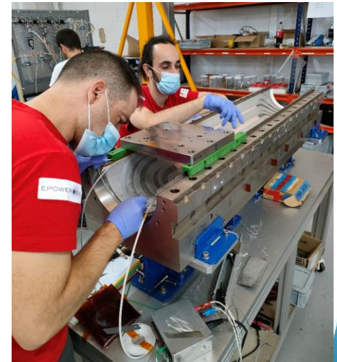
Impregnation mould assembly
