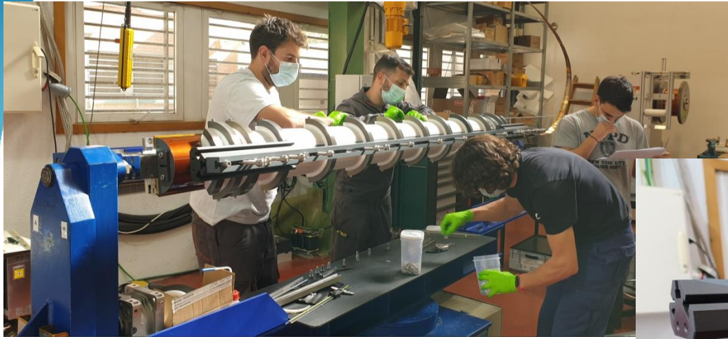
Inner layer winding
