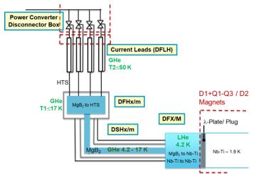
HTS cables in SC Link transport current from HL-LHC to tunnel
