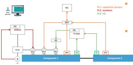
Mechanical bellow protection: 3 layers of protection (position sensors and interlock on motor)
