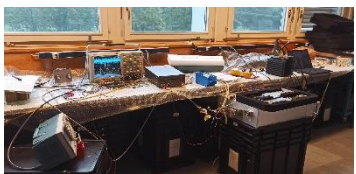
Electrical heaters tested with LN 2 before & after irradiation (>30 thermal cycles, 2 days testing)
