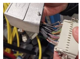
~2500 connectors and 25000 pins needed to acquire the signals
