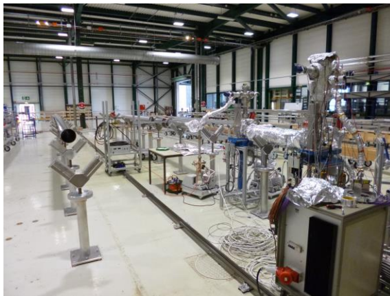
✓ 2 aC coating benches with chambers
