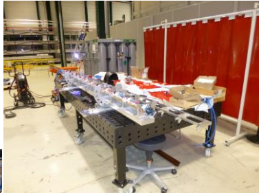
Tack welding of beam screen tube segments
