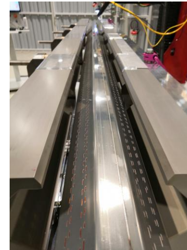
Longitudinal welding tooling
