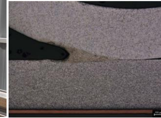
Metallography for the cooling tube weld qualification
