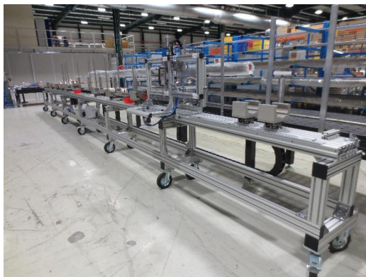
Dedicated bench for the stud welding of the absorber pin supports
