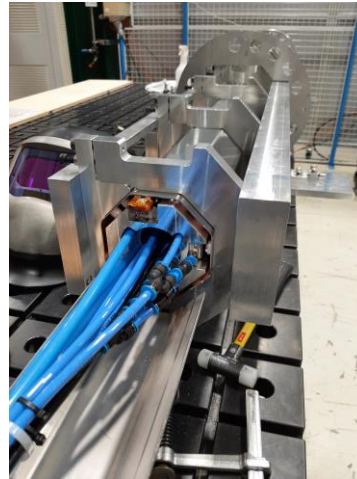
Tack welding tooling
