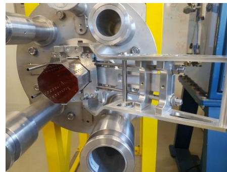
Cooling tube bending tooling (Q2 type)
