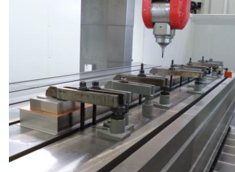
Machining to width and length
