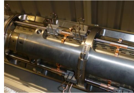
Beam screen assembly before laser weld
