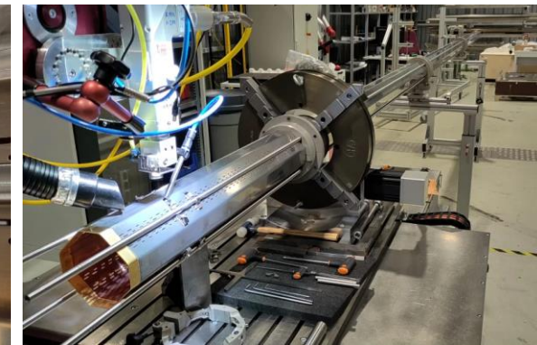
Welding of the contact rings, cooling tube supports and fixed points
