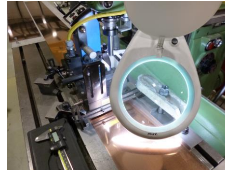
Copper removal at the edges
