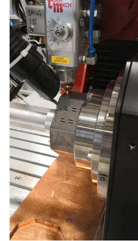
Cutting to length of the beam screen segments
