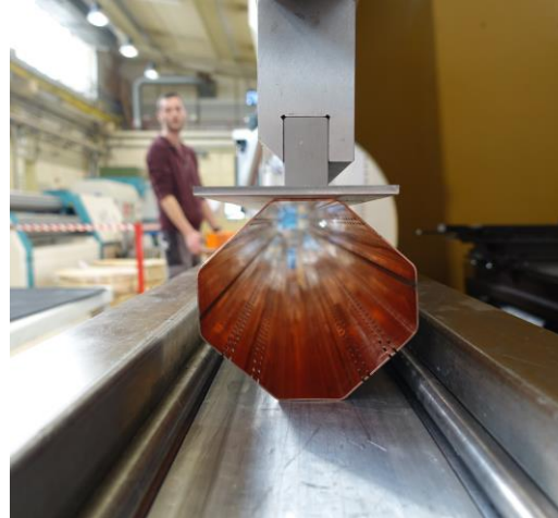
Calibration of the beam screen segments
