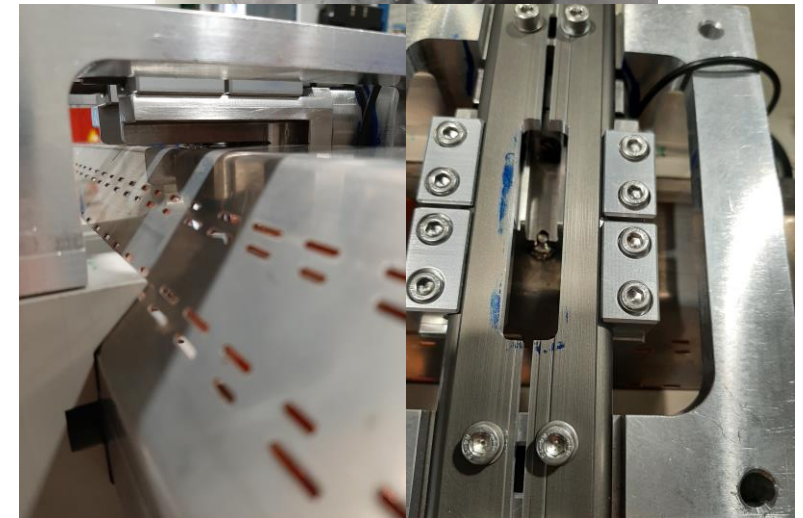
Tooling for stud welding quality check
