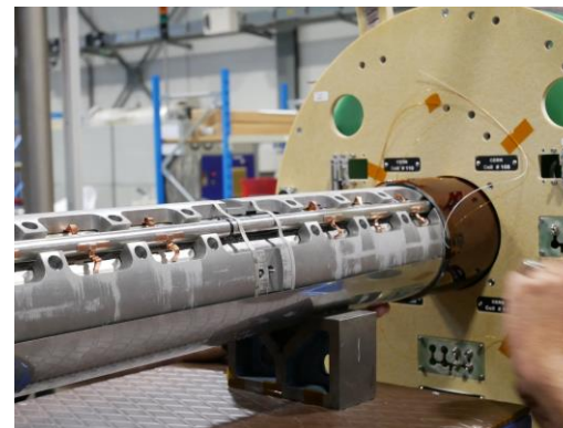
Prototyping and characterisation and validation tests in magnets (field quality and quench)
