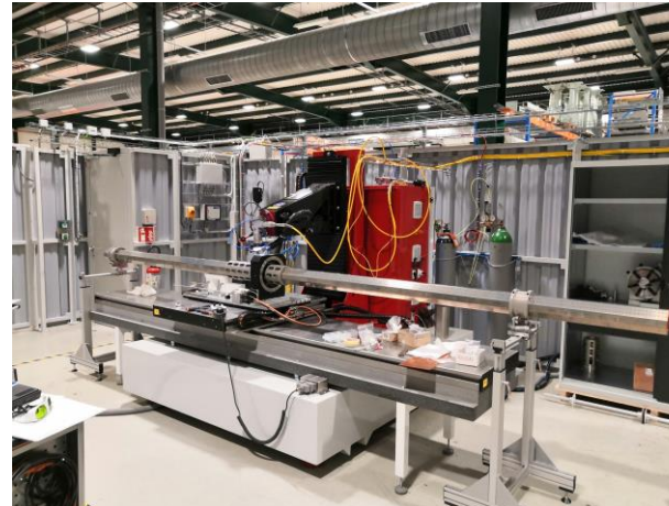
Butt welding of the beam screen segments
