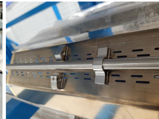
Welding of the contact rings, cooling tube supports and fixed points
