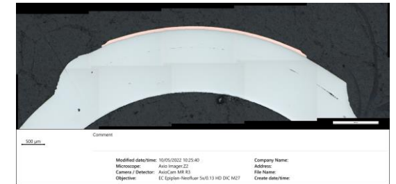
Metallography for the thermal link weld qualification
