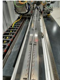
Laser welding bench for the cooling tube welding
