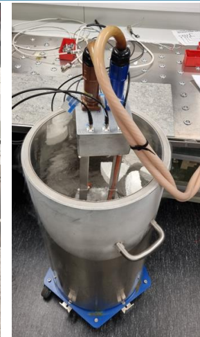
HL_LHC diodes: electrical tests at 300K and LN2
