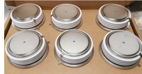
HL_LHC diodes: electrical tests at 300K and LN2
