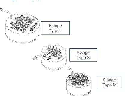
However, 6 prototypes flanges "Type L" of 48 HVs were produced and are used in the first Q1/Q3 magnets. Two prototypes flanges "Type S" of 18 HVs were also produced and will be used on first Q2 magnets. The IFS boxes are adapted accordingly.
