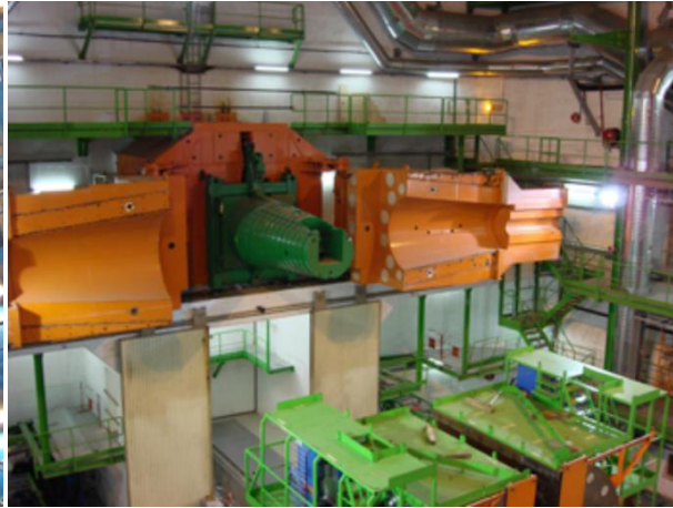
CMS Forward Shielding (rotating shielding + Fixed Iron Nose FIN)
