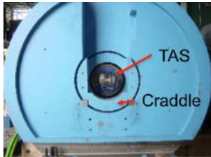
ATLAS Forward Shielding (here Monoblock TX1S insertion into Fixtube)
