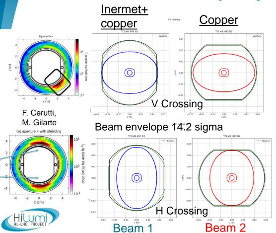
Present shape for both <u>Inermet</u> and <u>copper</u>: Round gap = 60.2+-1mm Flat gap = 50.6+-1mm
