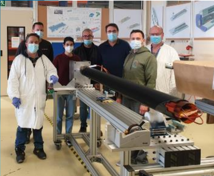
MCBRDP4 apertures and magnet assembly at 927 (SMT)
