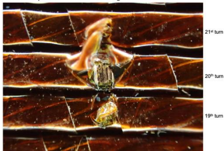
Fig. 3: Macrograph of insulation damage.
