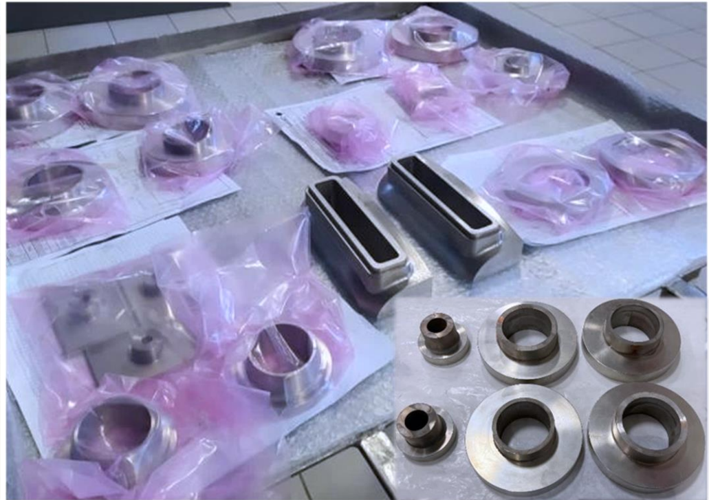
Sub-components & Brazed Joints ready for weld
