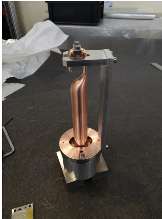
EB weld tooling for last weld
