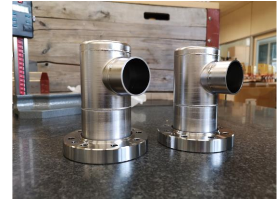
Nb Body with brazed 316LN flange
