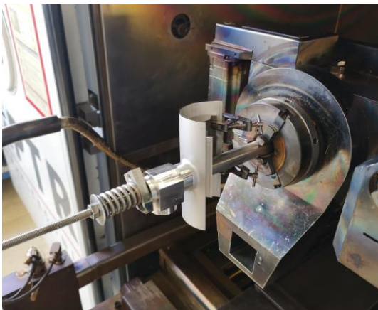
Vacuum brazing St. Steel to Nb Stainless Steel jacket welding
