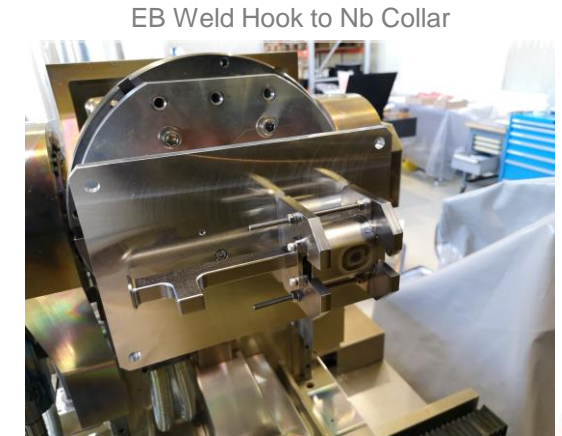
EB Weld Hook to Nb Collar
