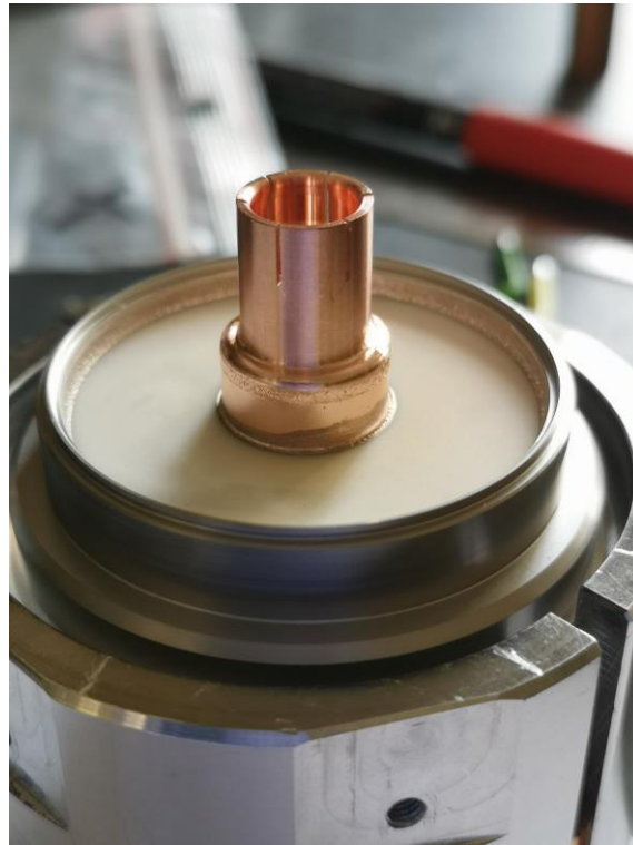
Brazed feedthrough with EBW RF clamp
